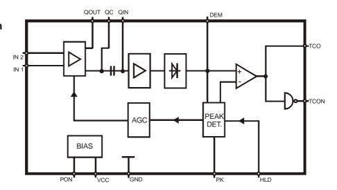
Figure 1. Block diagram
